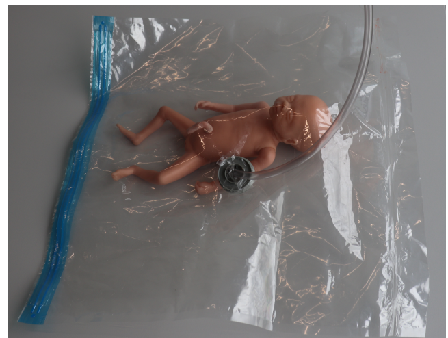
Figure 1. The prototype of the first variation: A model of a premature baby inside a transparent rectangular plastic bag.
